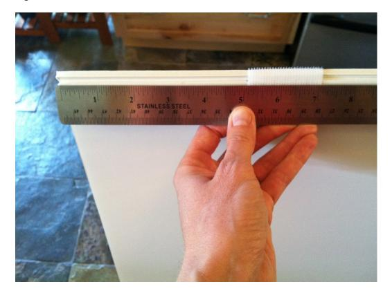
5. Measure 16" from the inside edge of the top soft piece toward the center and place another soft strip to hold the pieces of poster board together. Do the same for the other side. There are now 4 soft pieces holding the top of the poster board together (Lines on photo indicate location of soft Velcro strips).
