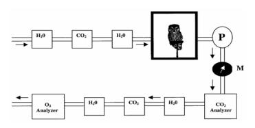
**Figure 3.** Generic arrangement of respirometry apparatus in a typical open-flow respirometry system for measuring oxygen consumption, carbon dioxide production, or both. Squares labeled  $H_2O$  and  $CO_2$  represent tubes containing materials for removal of water and carbon dioxide from the air, respectively. P is a pump and M is a flowmeter.
